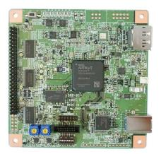
Windows and Linux. The board can operate on USB bus power. If the host PC does not have supply capacity enough, supply +5V from CN1.
